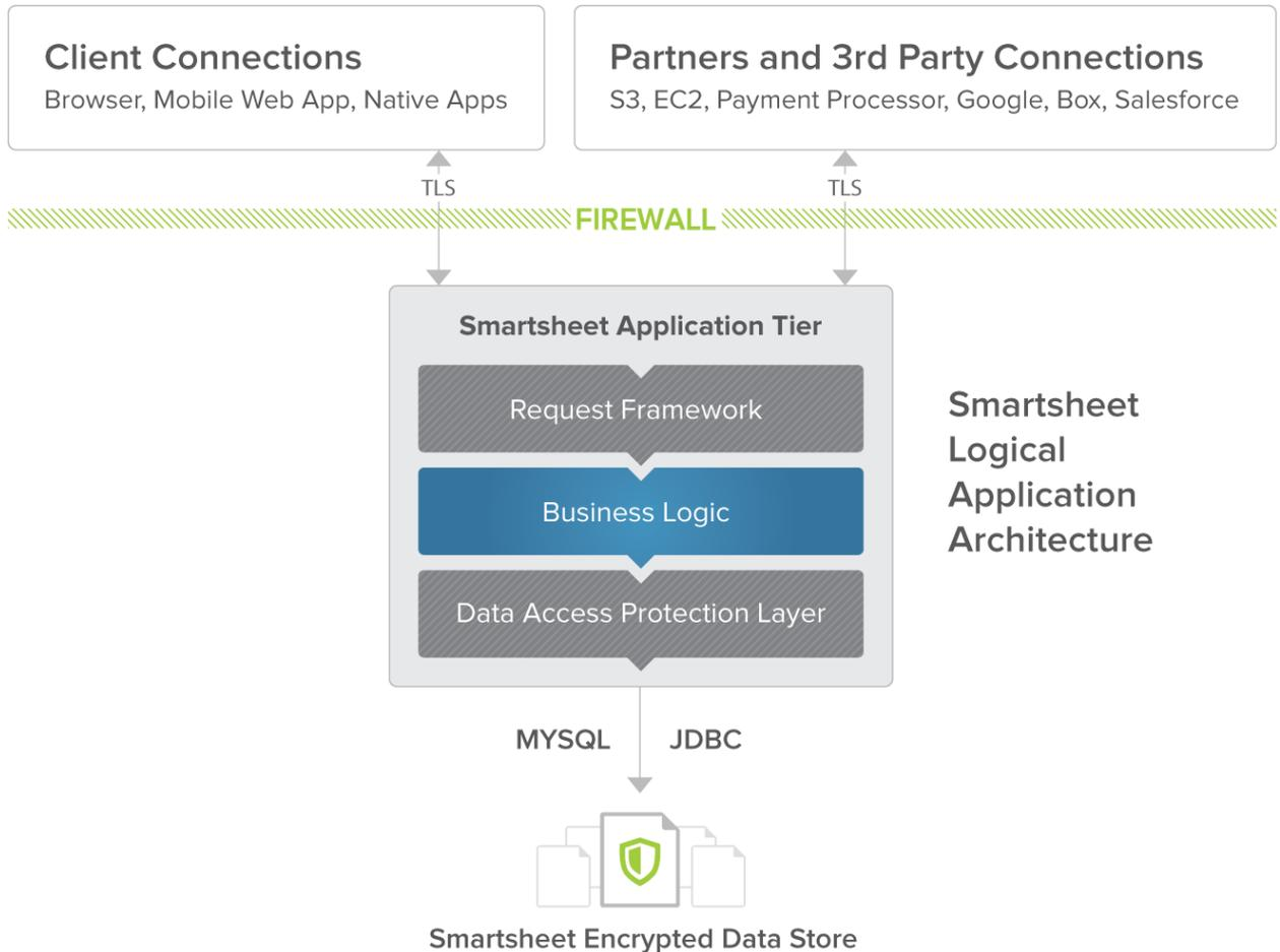
**Figure 1 – Logical Overview of Smartsheet Operating Environment**
